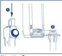
Slide rod down 1. Insert syringe into recess 2. **Adapter for** red syringe
