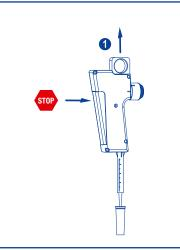
Trigger self-locking when remaining liquid is insufficient. Pull rod upwards to aspirate liquid 1.
