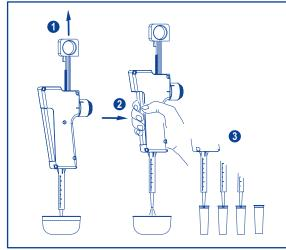
Slowly pull rod upwards to aspirate liquid (). Check absence of air bubble in liquid column. Press trigger in full, discard first shot 2. Depress trigger until stop and release completely for each aliquot 3.
