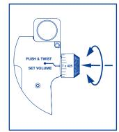
Press knob and simultaneously rotate until volume scale and setting mark are even.
