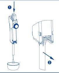
Push rod down to empty remaining liquid (). Slide syringe out of recess 2.
